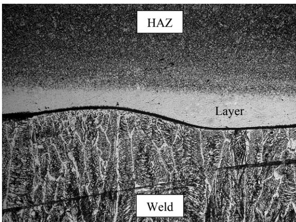
Fig. 3 – Overlaying with austenitic electrodes Fox CN 23/12 Mo-A on a plate of P91 steel after tempering 750 °C, 18 h, magnification x100
