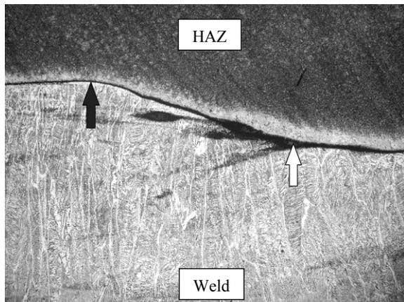
Fig. 2 – Convexity and concavity of a large radius of curvature (white arrows indicates increased decarburization in HAZ, dark arrow – reduced decarburization in HAZ), magnification x50
