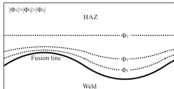
Fig. 5 – Requirements for the obtained values of some function  $\Phi$  at HAZ points for estimating the distance and local curvature of the fusion line
