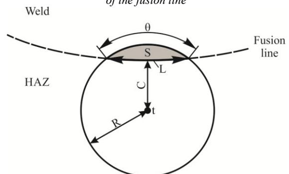
Fig. 6 – Geometric interpretation of parameters  $L$ ,  $R$  and  $\theta$
