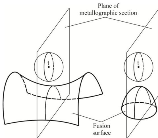
Fig. 9 – Hyperbolic and elliptical paraboloids having the same parabolic cross section, but different values of  $\Phi(t)$
