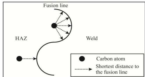
Fig. 4 – Scheme of the possible mechanism of influence of the fusion line geometry on the diffusion of carbon
