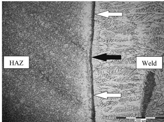
Fig. 1 – Convexity of small radius of curvature (white arrows indicates increased decarburization in HAZ, dark arrow – reduced decarburization in HAZ), magnification x200
