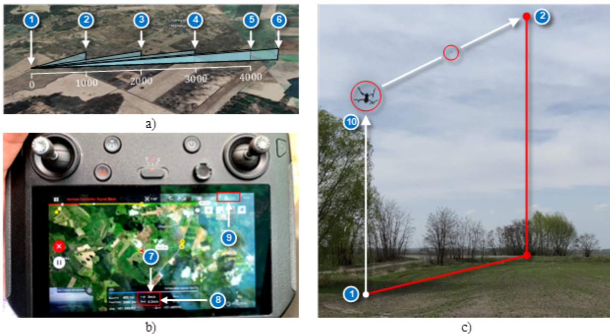
Fig. 9 – Experiment: (a) Flight route of the drone on Google Maps; (b) evaluated parameters on control panel; (c) photo of the drone flight path to the observation point according to the third flight profile; where 1 – launching site, 2...6 – observation points (1000, y_D ), (2000, y_D ), (3000, y_D ), (4000, y_D ), (4500, y_D ), respectively, 7 – S_{ver} , 8 – S_{hor} , 9 – SOC, 10 – altitude of 10 m.
