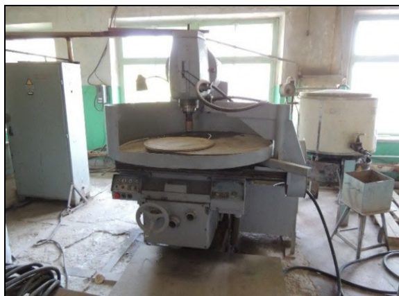
Fig. 2 – A horizontal milling machine for glass balk grinding
