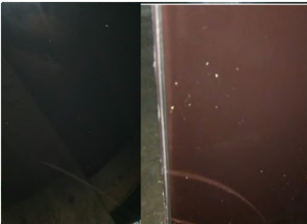
Fig. 4 – Color differences in glass-ceramic enamel after firing due to application on the tin and air sides of the glass
