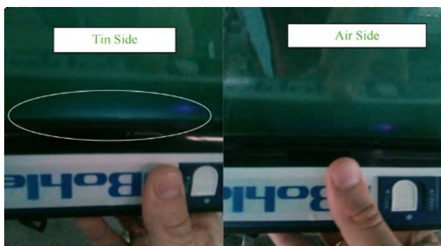
Fig. 2 – Difference between the tin and air sides under ultraviolet illumination
