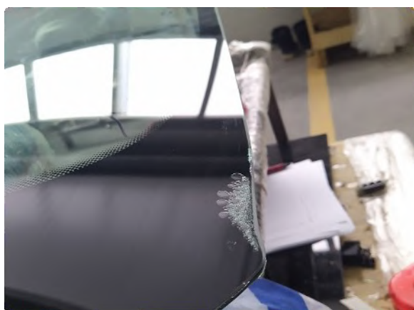
Fig. 6. – Result of not correct bending process after autoclaving stage
